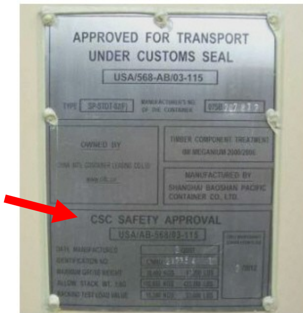
CSC ID Plate: Revised standards in 1993 by CSC. Transport seal combined with CSC Certification.
