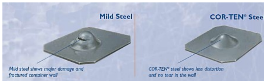
TEST: Corten steel used on shipping containers is virtually undamaged (Cronos)
