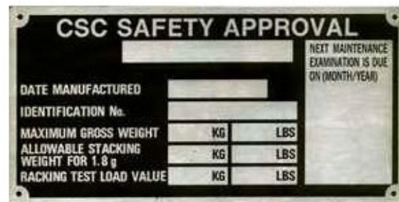
CSC ID Plate: Not combined with Transport seal.
